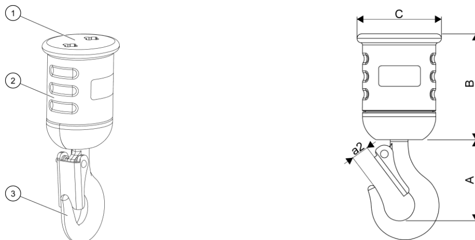
Figure 28. Two-fall (2/1) hook block for frame sizes CA1–CB1
